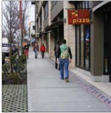
This streetscape is designed with pervious paving, street trees and other planting—types of green stormwater infrastructure.
