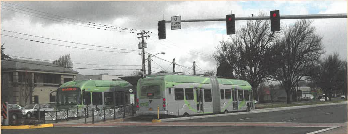
EmX in Eugene, OR operates along a dedicated center running transitway.
