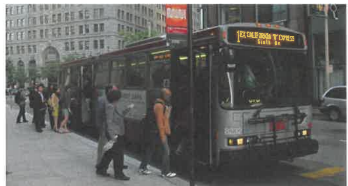
All door boarding on Muni's 1BX Express line in San Francisco reduces dwell time at stops.
