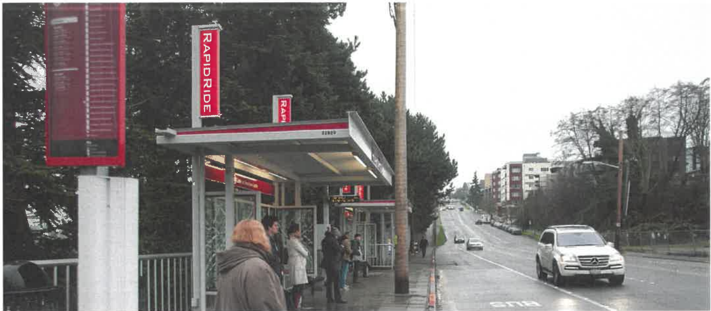
Fully featured RapidRide stations include shelters, benches, tech pylons with real time information, off-board payment validation, system maps, and branded signage. Image from King County Metro
