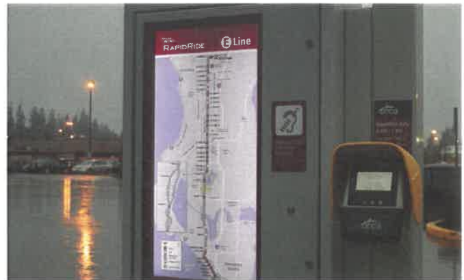
RapidRide tech pylons provide real time information, system maps, and off-board ticket validation.
